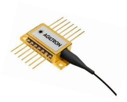
The 730nm series laser diodes are fabricated in a hermetically sealed 14-pin butterfly package. The laser diodes contain a monitor photodiode, thermoelectric cooler (TEC), and a thermistor to secure high-quality laser performance. Our laser products are Telcordia GR-468 qualified and in compliance with RoHS Directives.
